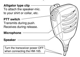
**NEVER** immerse the connector in water. If the connector becomes wet, be sure to dry it BEFORE attaching it to the transceiver.
